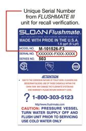
The manufacturing date code/serial number is 16 characters long and is located on the label on the top of the Flushmate System's polypropylene vessel. The first six numerals of the serial number are the manufacturing date code. The manufacturing date codes for the affected Flushmate Systems begin with 101497 (October 14, 1997) and continue through 043011 (April 30, 2011).
